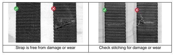
• All anchoring points for rigging (straps) must not have an abrasive surface or sharp edges. Strap damage can lead to a serious injury (even lethal).
